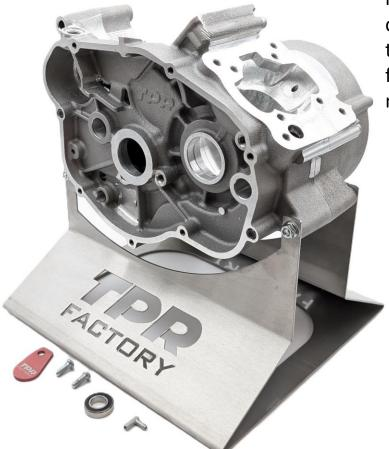
Already prepared to ALLOW 47 mm stroke crankshafts and Ø52 cylinders installation with through studs. In addition, flanged cylinders can also be mounted on it.
